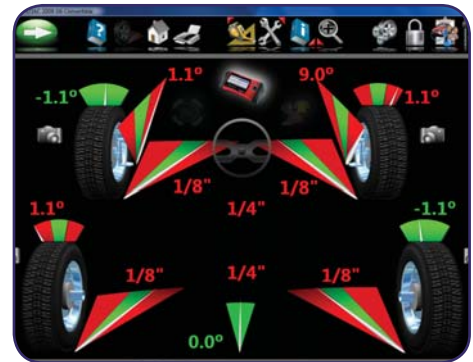
3 Obtain all alignment readings in under 2 minutes. Adjust vehicle using live measurements.
